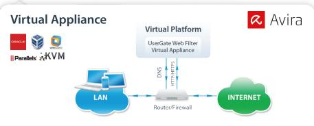
UserGate Web Filter Virtual Appliance is supplied in OVF (Open Virtualization Format) supporting such vendors as VMware, Oracle VirtualBox, Parallels and KVM. UserGate Web Filter Virtual Appliance is a special disk image for deployment UserGate Web Filter on virtual machine.
