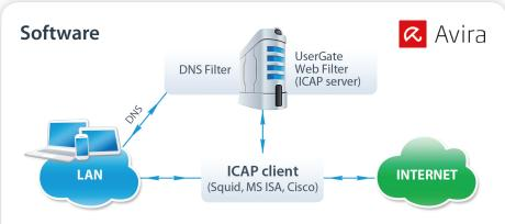
UserGate Web Filter can perform filtering at the level of DNS and HTTP/HTTPS requests. When filtering DNS requests, UserGate Web Filter emulates a DNS server with extensive filtering capabilities.
